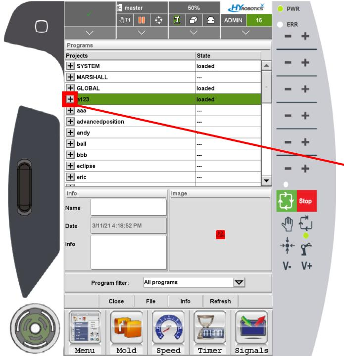
Press + button and Expand currently loaded mold project file
